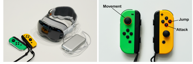
Figure 3: The hardware used in the user tests. Apple Vision Pro headset and Nintendo JoyCons (left) and the control scheme of the Controller condition (right).
