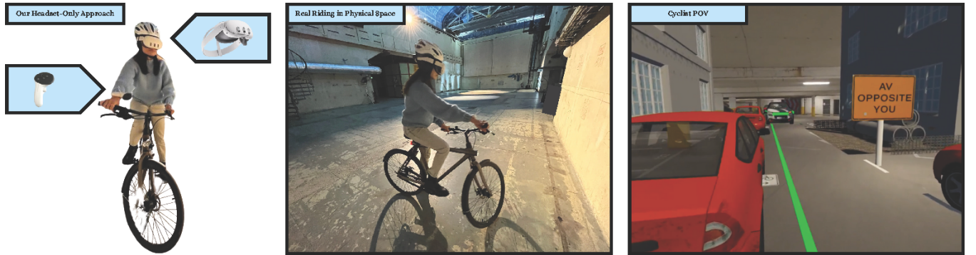
Figure 3: Study Setup. Left: Our headset-only approach with the left controller on the participant's wrist to simulate a smartwatch. Middle: A cyclist riding in real physical space with a mixed-reality headset. Right: The cyclist's point-of-view, with the real world (the indoor hall) overlaid with to-scale AR objects, in this case, the FullIntel interface in one of our scenarios.
