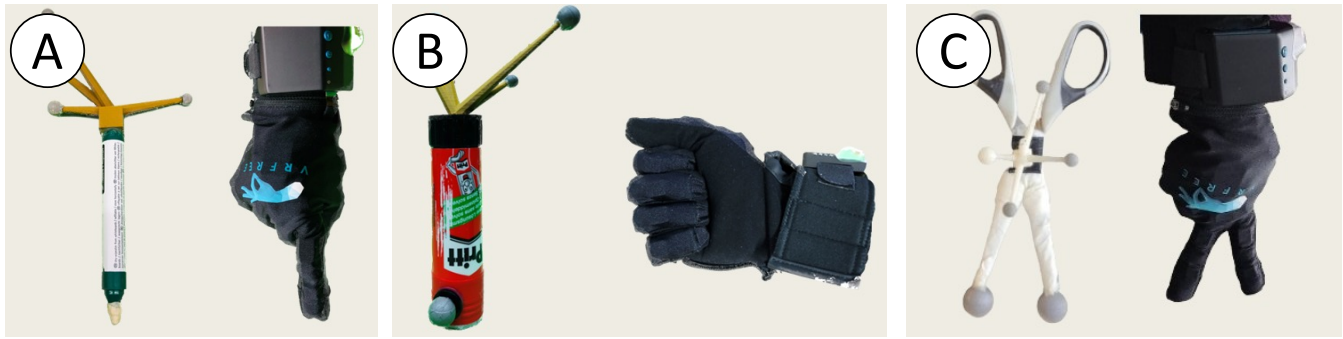
Figure 2: Proxy- (left) and gesture-based (right) techniques are used in VRPaperCrafting for (a) coloring, (b) gluing, and (c) cutting. To use physical objects in VR, we augmented them with Optitrack markers placed on 3D-printed add-ons. To enable hand gestures in VR, we used VR gloves by Sensoryx and a pointing gesture to enable a pencil, a fist gesture to start a gluing stick, and a two-finger (scissor-like) gesture to activate scissors.
