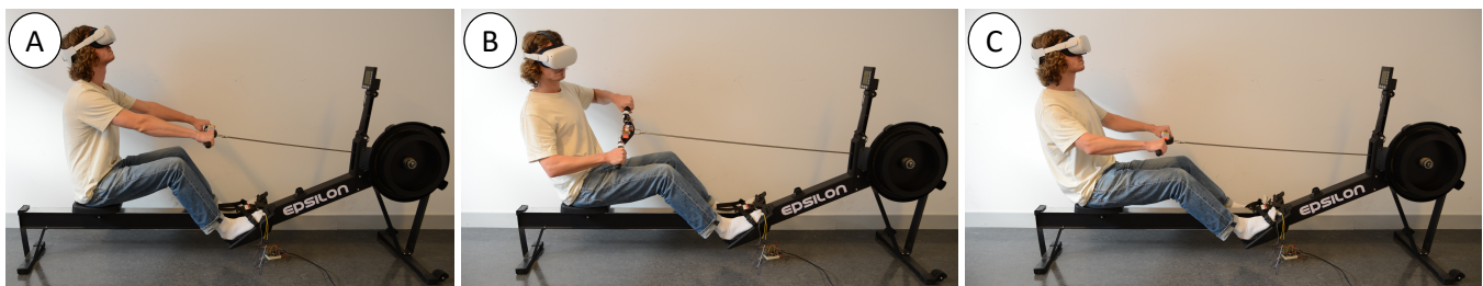
Figure 1: The three steering methods for rowing-based locomotion: (a) head-based steering indicates the direction of movement according to the head's orientation, (b) hands-based steering employs handlebar rotation on a 2D plane and buttons under thumbs to go up and down, and (c) feet-based steering is based on the pressure distribution between left and right feet for steering on a 2D plane and between toes and toes joints for steering in a 3D space.
