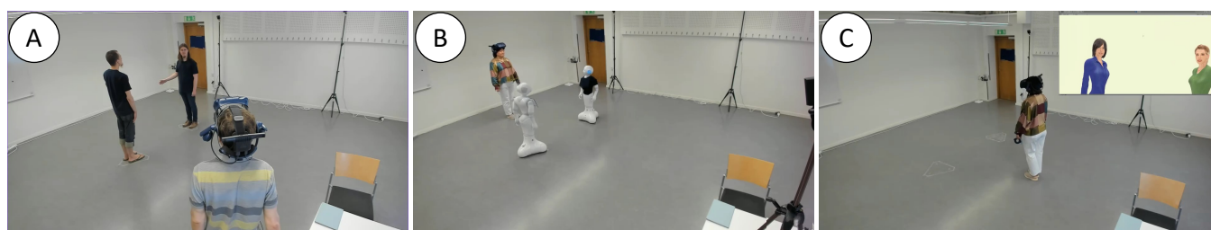
Figure 1: Overview of setups with three different types of embodiment, in which participants had to join a group of: (A) humans, (B) robots, and (C) virtual characters. Only in scenario C, participants were fully immersed in VR, while in A and B, they wore the VR headset for tracking purposes and it was not positioned directly in front of their eyes. The participant is standing at the starting position (A), the participant joined at the furthest side of the group (B), and the participant joined at the closest side (C).
