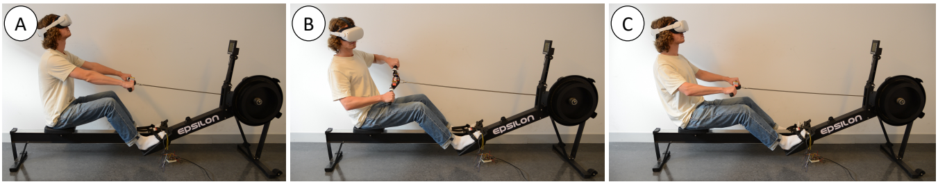
Figure 3: We investigated three steering methods for rowing-based locomotion: (a) head-based steering indicates the direction of movement according to the head’s orientation, (b) hands-based steering employs handlebar rotation on a 2D plane and buttons under thumbs to go up and down, and (c) feet-based steering is based on the pressure distribution between left and right feet for steering on a 2D plane and between toes and toes joints for steering in a 3D space.
