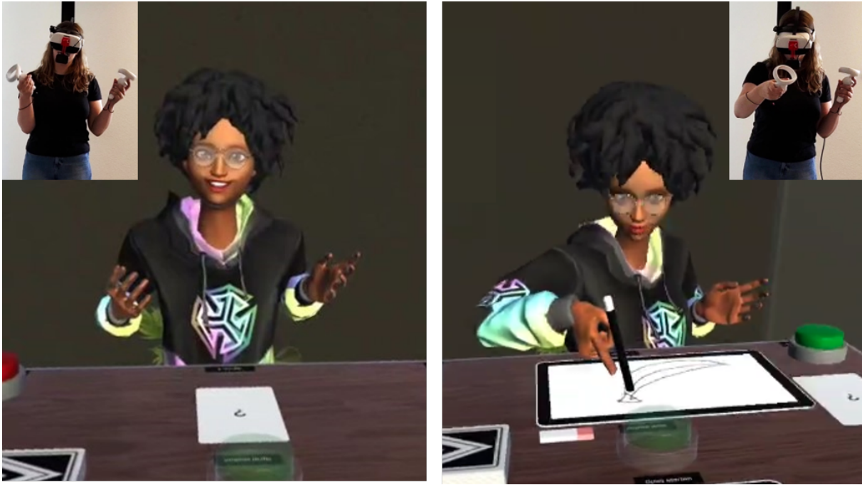
Figure 2: User in the real-world environment wearing VR glasses and the avatar embodying her in both types of explanation. The avatar portrays the user’s eye movements (gaze direction, degree to which eyes are opened) and mouth movements (position of various mouth landmarks) while performing verbal explanation (left), and the avatar shows neutral facial expression in graphical explanation (right).
