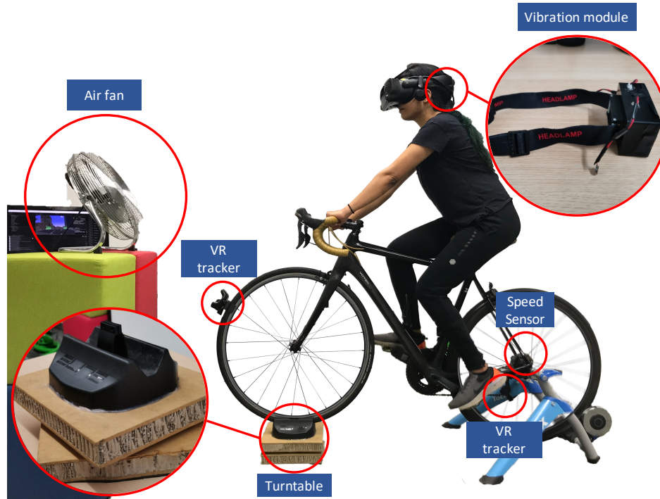
Figure 4: Experimental setup used in both studies: Participants cycled on a stationary bicycle simulator while wearing a VR head-mounted display. The VR trackers and the turntable were used to measure the rotation angle of the handlebar and speed sensor – the cycling speed. In the second study, additional countermeasures against VR sickness were used: a fan placed in front of the head, vibrotactile feedback integrated into the head-mounted display behind the ears, and a reduction in the field of view displayed in the HMD. Another difference between study 1 and 2 is in the bike platforms: The figure shows the Tacx platform used in Study 2, while Study 1 used the Kinetic Rock and Roll to facilitate upper body movements.
