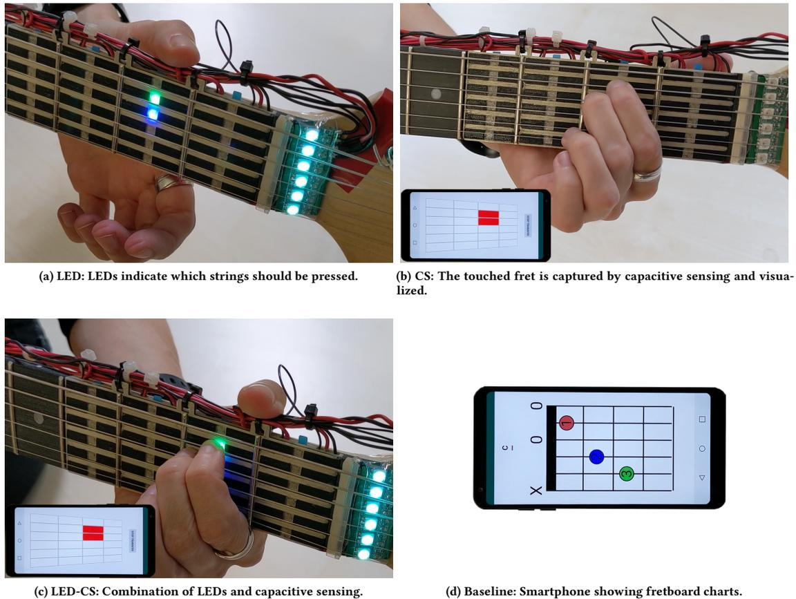
(a) LED: LEDs indicate which strings should be pressed.
