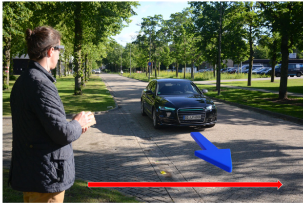
Figure 2: Experiment setup: The pedestrian stands on the edge of the road on the pavement wearing a mobile eye tracker and holding the slider input device and indicates their willingness to cross in real time as the AV approaches them. The blue and red arrows represent the path of the AV and the pedestrian respectively.
