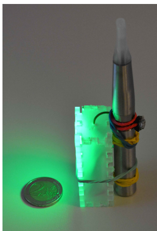
Figure 3: Our early VapeTracker prototype (attached to the Joyetech ® eGo-C e-cigarette) emitting green ambient light, placed next to a €2 coin for size comparison.
